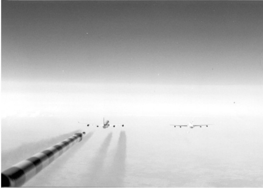
Figure 7. Photo of an Airbus A340 with contrails (left) and a Boeing B707 without contrails (right) at 10.5 km altitude taken from the Falcon cockpit [36].
